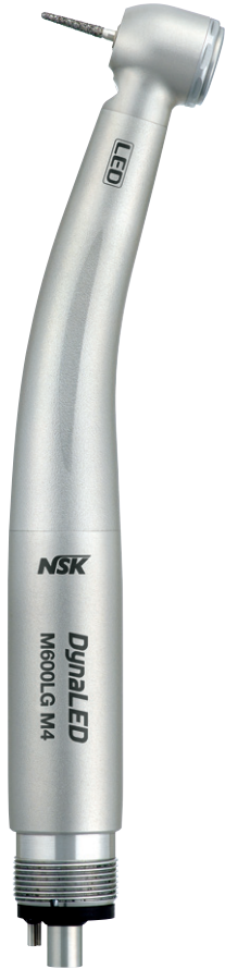
Miniature Head Power : 15 W (M4, B2) / 13 W (QD) Speed : 380,000-450,000 min -1 Head Size : ø10.6 x H 12.4 mm, 25,000 LUX *Both standard and short shank burs are applicable.
